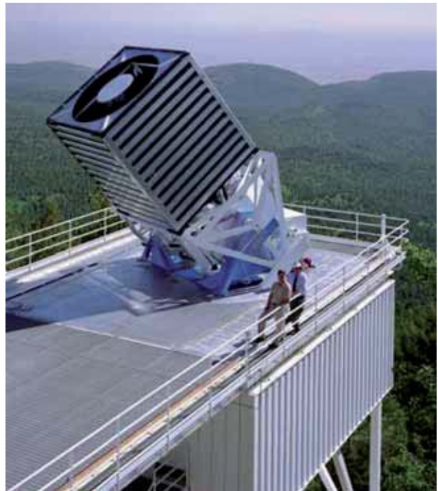
The Sloan Telescope, a 2.5-meter telescope at Apache Point Observatory, did all SDSS imaging and spectroscopy. picture: The Sloan Digital Sky Survey.
